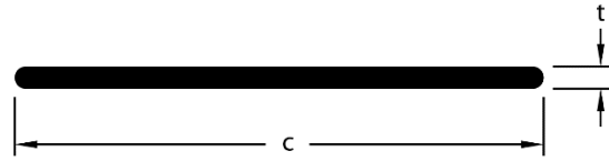
Figure 4-28- The schematic of the simplified 2D airfoil shape.
